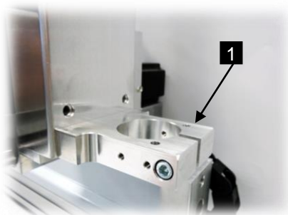
Abb. 11: Tool holder 43H7
