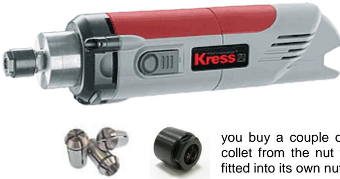
The Kress uses a collet system to support various shank diameters of tooling. The Kress itself comes with an 8mm collet, though we recommend the Kress collet set along with your machine order to support more of the standard small tool sizes.
