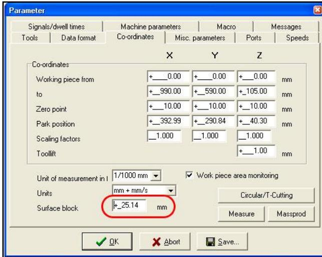
To enter this sensor activation height value, navigate to the 'Parameters > Co-ordinates' menu and enter in the height value into the 'Surface block' entry. Then save and exit and you're ready to go.
